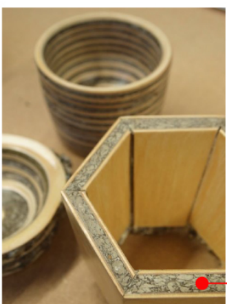
Compressed and dyed 'paper-ply' from office waste (Jack Scott BA 3D)
