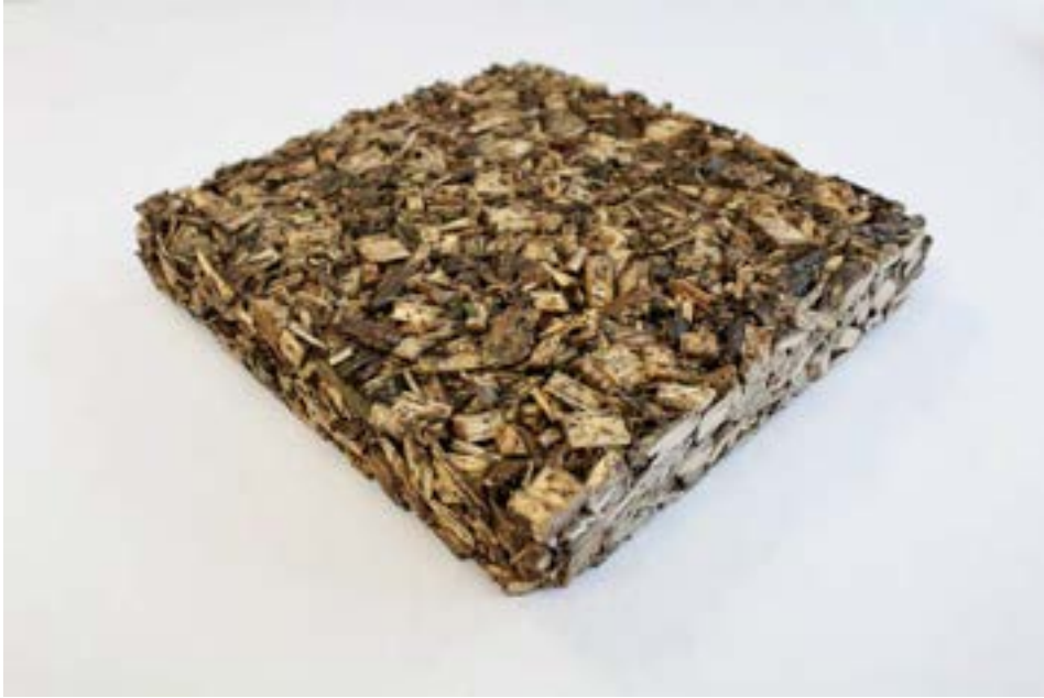
Chipboard made from waste from door prototype waste and pine resin. Image: Nick Gant, 2023
